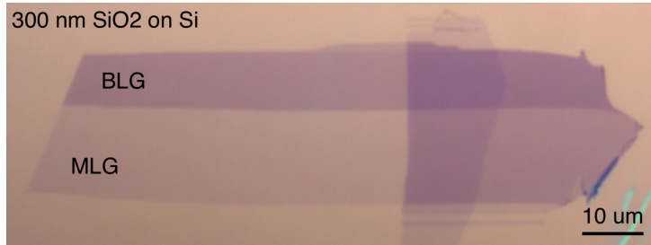
(a) Optical photo of monolayer graphene (MLG) and bi-layer graphene (BLG) on silicone substrate.
